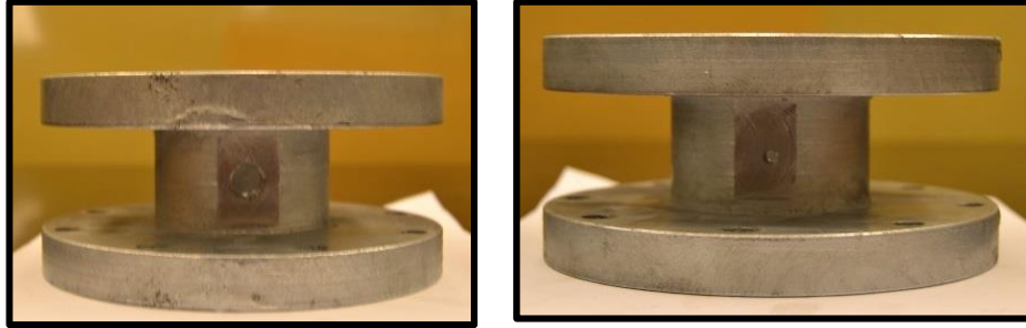
Figure I: Left: the gas inlet port. Right: The pressure microphone port and how the resonator surface is flattened to provide proper sealing
